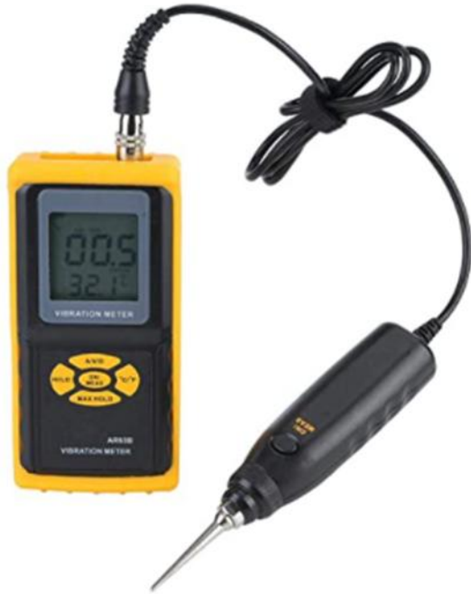
Photo 5 - AR63B Vibration Meter
